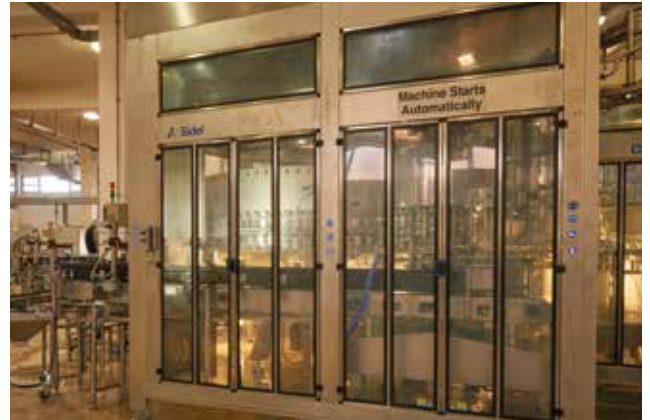
The new electronic volumetric type filler ensures consistent product fill volumes irrespective of bottle size.
