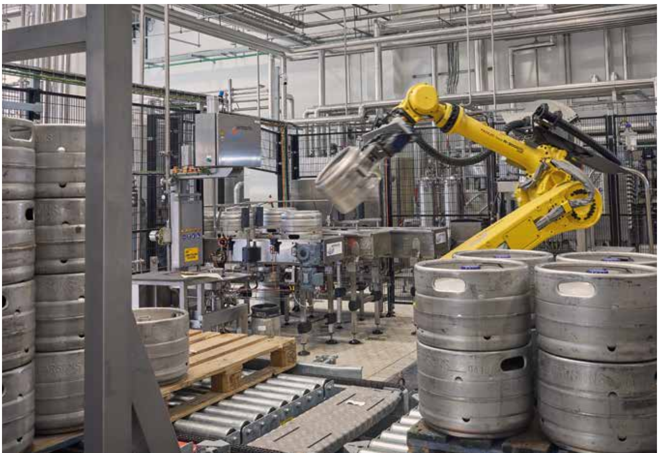
The dedicated robotic arm, handling both empty and full beer kegs.
