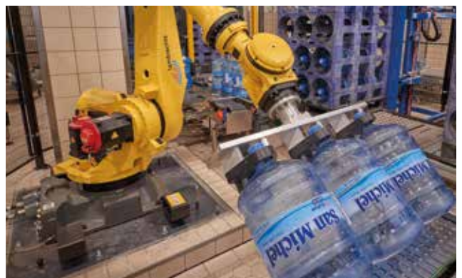
The EcoPure robot unloading empty 18.9 litre bottles onto the infeed conveyor of the table water line.
