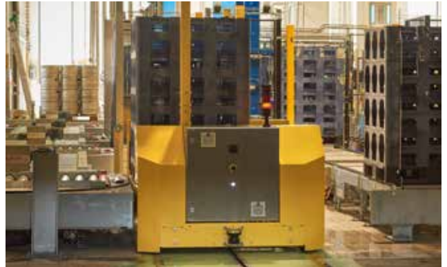
Fully automated handling of pallets by the Automated Guided Vehicle.
