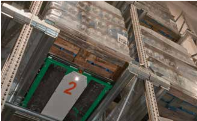
The semi-automated Radio Shuttle device moves pallets for storage into the new density racking system.
