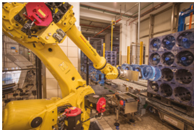
The EcoPure robot stacking 18.9 litre bottles in crates
